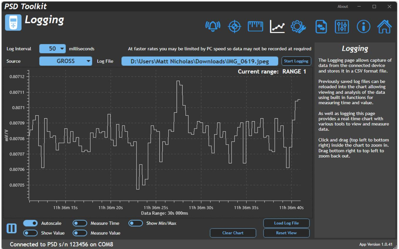
This page allows data from the handheld to be logged to a file and later reloaded to be viewed on the chart. A real-time chart is always visible whether logging is active or not.
