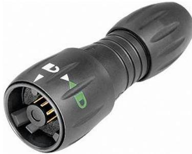
To attach this connector to the handheld, align the white arrow on the connector with the white line on the handheld socket then rotate the locking collar as indicated on the connector.
